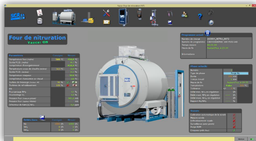
SCADA - SCR supervision system
